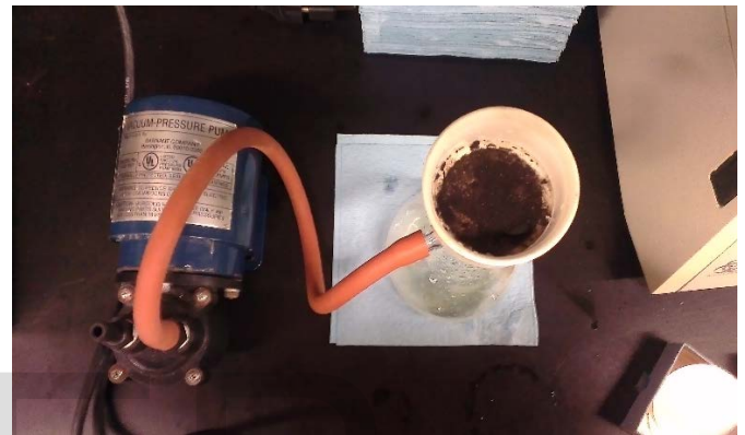
Figure 9: Vacuum pump setup to remove suspended particles
