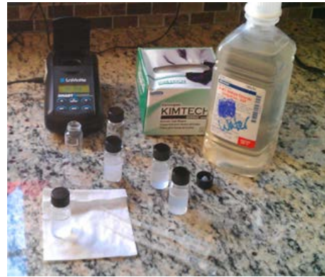
Figure 8: LaMotte SMART 2® colorimeter to detect nutrient levels
